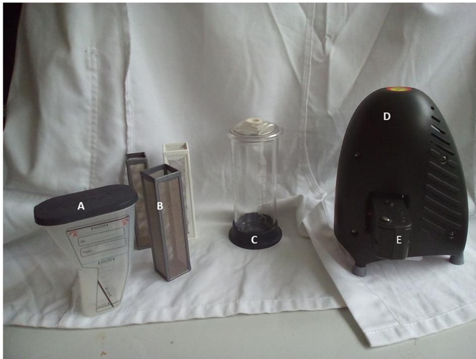
**Figure 1.** The supplied FECPAK<sup>G2</sup> equipment. A: Sedimentor; B: 1 mm white pre-filter and 600 and 425 µm silver filters; C: filter cylinder; D: Micro-I imaging device; E: FECPAK<sup>G2</sup> cassette, inserted into Micro-I.
